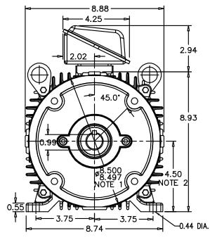
NOTE 1: C-FACE & TACHOMETER MOUNTING
