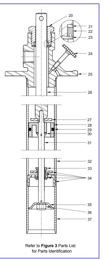
Figure 4 Pump Tube Assembly 332810- Section View
