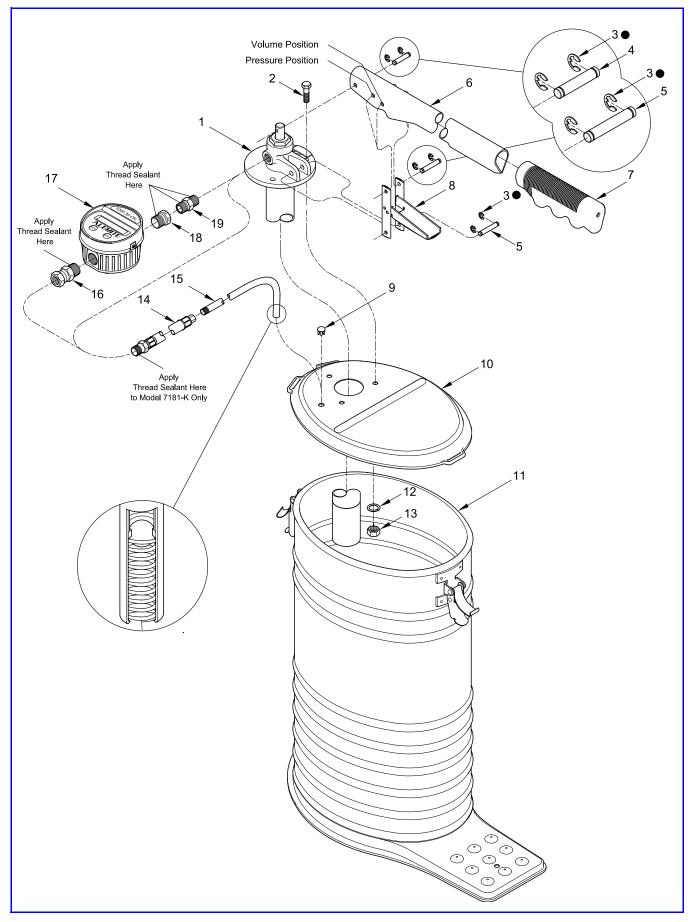
Figure 2 Portable Hand-Operated Pump Model 7181 Series - Exploded View
