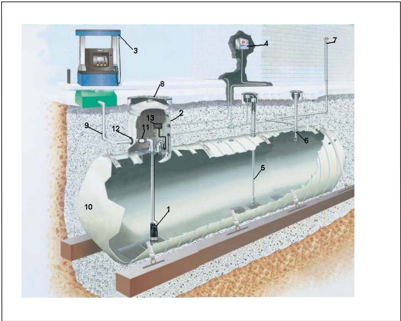
Figure 2 8427 - Typical below ground installation
