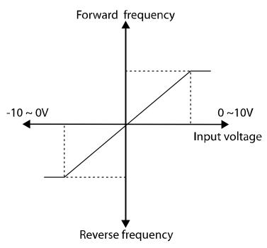
[Bipolar input voltage and output frequency]
