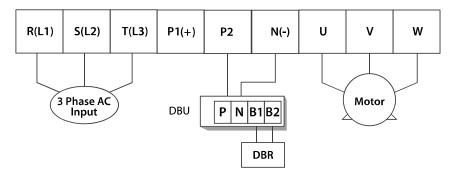
In 30-75 kW 200 V model types, the P1 and P2 terminals are connected with a jumper pin.
