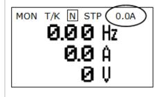
Ensure that the unit in the status display is changed to amps (current) in Monitor mode.
