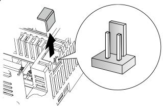
Connect the two jumper pins using a short circuit connector to activate the EMC filter. 3
