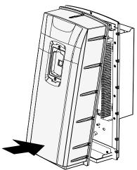
2 Insert and tighten the screws. There are 9–13 screws on the cover depending on the model type.
