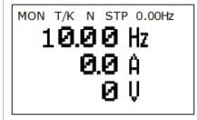
The frequency reference is set to 10 Hz.
