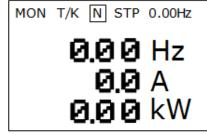
Ensure that the third displayed item in Monitor mode is changed to the output power.
