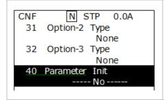
The Parameter Initialization option is displayed again when the initialization is complete.
