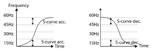
[Acceleration / deceleration S-curve pattern configuration]
