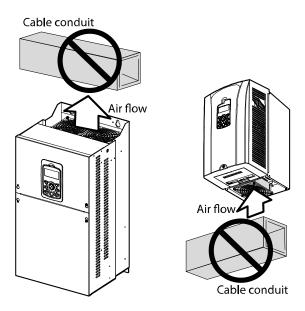
Ensure sufficient air circulation is provided around the inverter when it is installed. If the inverter is to be installed inside a panel, enclosure, or cabinet rack, carefully consider the position of the inverter's cooling fan and vents. The cooling fan must be positioned to efficiently dissipate the heat generated by the operation of the inverter.
