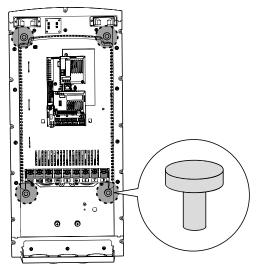
Place the inverter on a flat wall or in a cabinet, and use 4 screws or bolts to securely fix the inverter to the surface.
