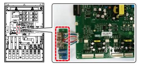
Refer to the following figure and install the safety board to the main SMPS board of the inverter using cable connectors.
