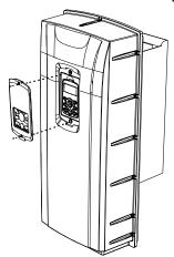
Depress the tab at the top of the keypad and gently lift the keypad from the inverter to remove it. 2 Be careful not to damage the keypad cable.
