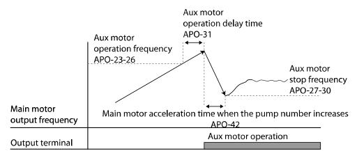
Auxiliary motor operation sequence by increased load
