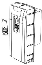
Depress the tab at the top of the keypad and gently lift the keypad from the inverter to remove it. Be careful not to damage the keypad cable.
