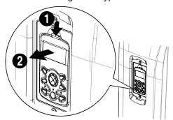
Depress the tab on the keypad cable connector and disconnect the cable from the back of the 3 keypad.
