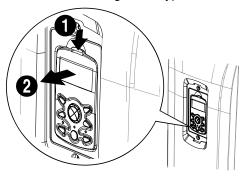
Depress the tab on the keypad cable connector and disconnect the cable from the back of the 3 keypad.
