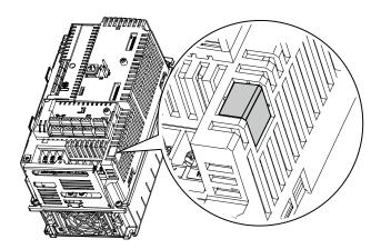
2 Remove the knockout cap and locate the jumper switch. The EMC filter will be deactivated if the two jumper pins are not connected.
