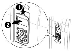
2 Depress the tab on the keypad cable connector and disconnect the cable from the back of the keypad.
