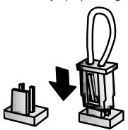
To remove the short circuit connector and deactivate the EMC filter, pull the connector while pressing the latch on the side of the connector. Use pliers or tweezers if you cannot reach the latch with your fingers.
