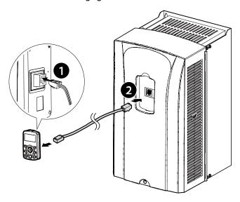
If a "Line Check" message is displayed on the keypad display and the keypad is not operating correctly after installing the remote cable, check the cable connection on both sides.
