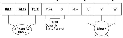
Connect the cables from the dynamic braking unit to the P (+) and B terminals to utilize the built-in dynamic braking unit.
