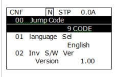
Press the [MODE] key to move to Configuration (CNF) mode.
