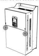
Slide the cover downwards and remove it from the inverter.
