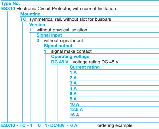
Description of ESX10-T signal inputs / outputs (see wiring diagrams).
