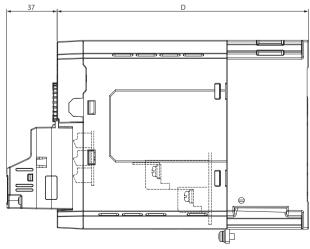
When mounting the communication option on WJ-C1, the D (depth) dimension is increased by 37mm. Take care when the communication option on WJ-C1 is installed in the cabinet.
