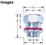
**Download Photo Image** Dimension A in Inches: .250-.350 Dimension B in Inches: .640 Dimension C in Inches: 1.210 Dimension D in Inches: .975 Dimension E in Inches: 1-5/16 Dimension F in Inches: 13/16
