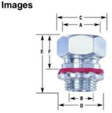
**Download Photo Image** Dimension A in Inches: .650-.750 Dimension B in Inches: .845 Dimension C in Inches: 1.440 Dimension D in Inches: 1.220 Dimension E in Inches: 1-9/16 Dimension F in Inches: 1-1/32
