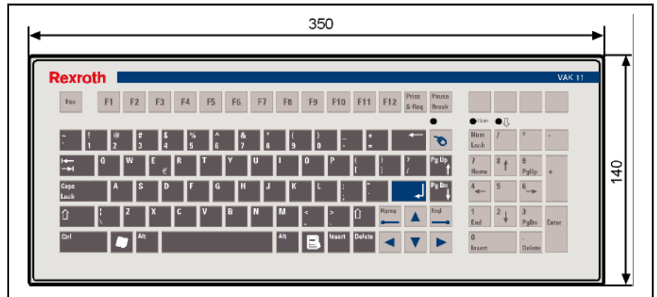
Fig.5-1: Housing dimensions VAK 11.2
