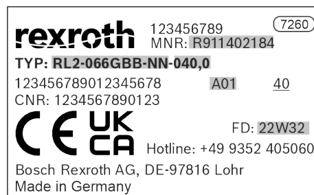
Fig. 7: Example of cable type plate
