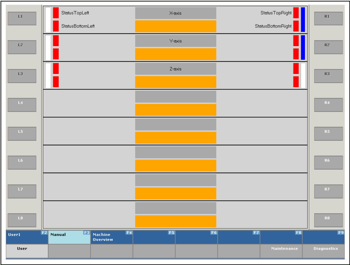
Fig. 4-23: Operating screen Depending on its configuration, an operating screen may contain 5 or 7 operating lines.
