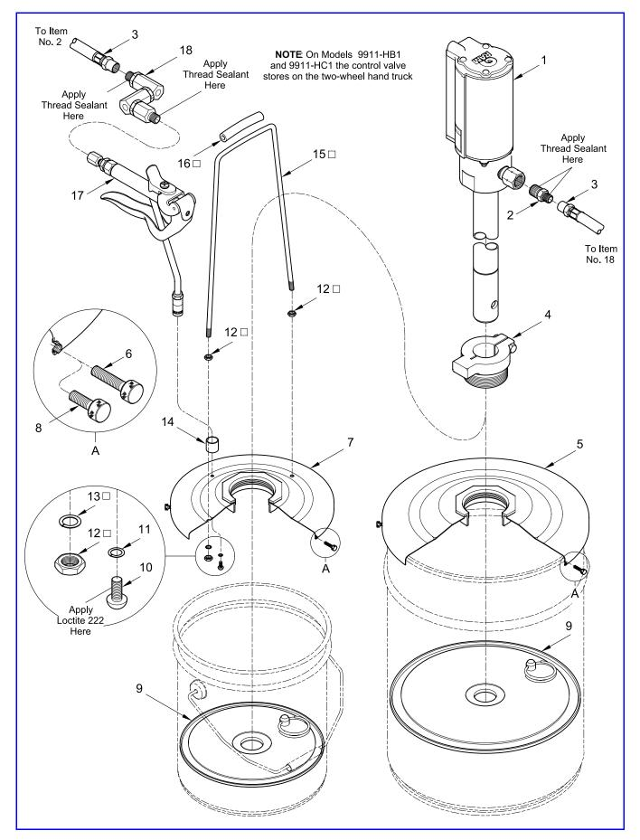
Figure 2 High-Pressure Portable Pump Models 9911-H1 Series - Exploded View
