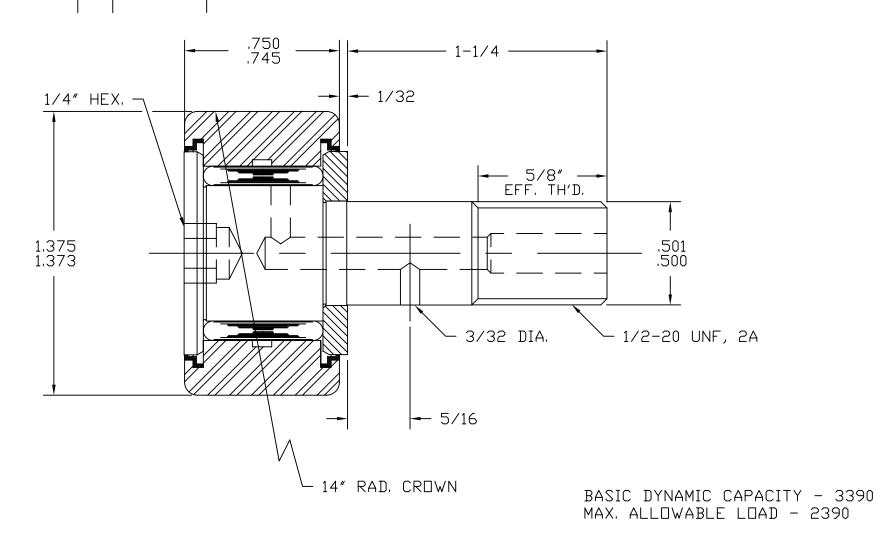
MAT'L: ST'D BEARING STEELS, SEALS - ACETAL. BEARING PACKED WITH GENERAL PURPOSE EP GREASE. RELUBE PROVISIONS WILL ACCEPT 3/16" DRIVE TYPE FITTINGS, PLUGS SUPPLIED FOR UNUSED HOLES. TOLERANCES
