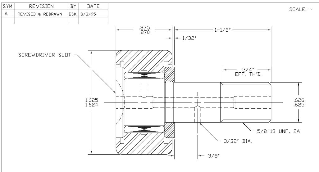
BASIC DYNAMIC CAPACITY - 4450 MAX. ALLOWABLE LOAD - 3760
