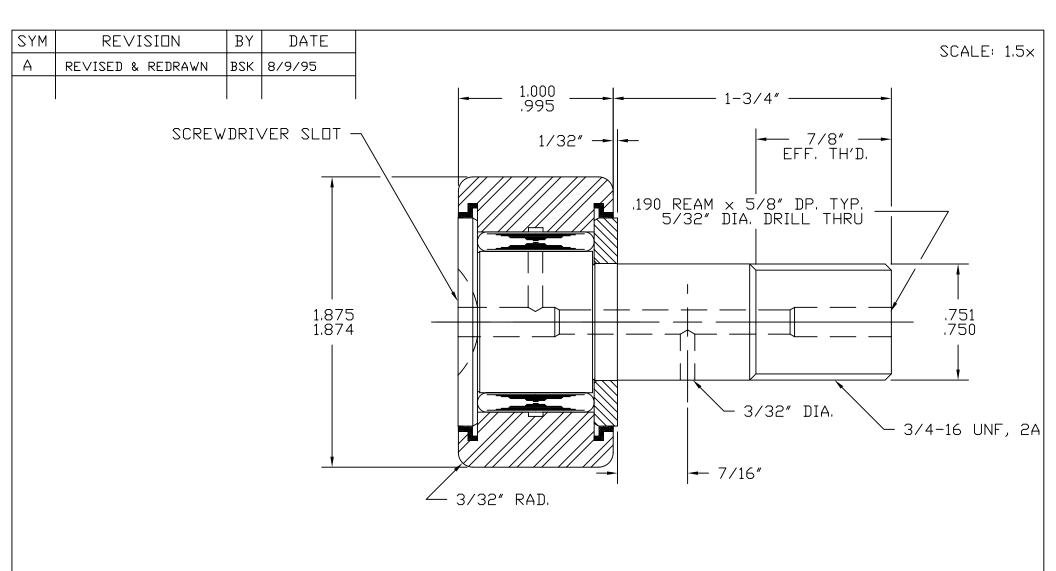
BASIC DYNAMIC CAPACITY - 6070 MAX. ALLOWABLE LOAD - 5400
