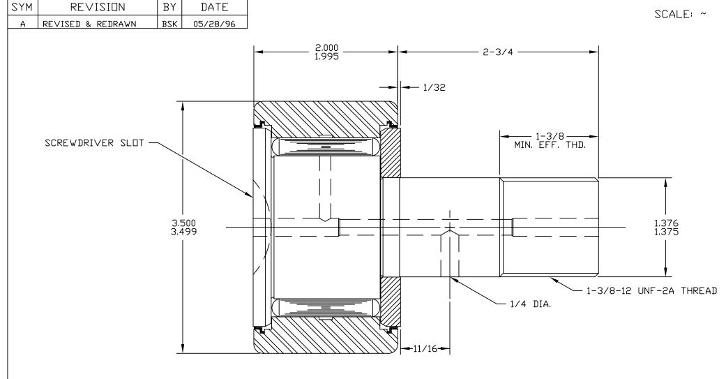
BASIC DYNAMIC CAPACITY - 22050 MAX. ALLOWABLE LOAD - 18700
