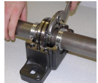
Figure 2) Tighten Until Snug
