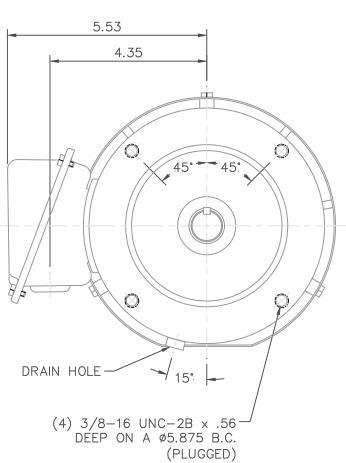
MAXIMUM FACE RUNOUT TO BE .004 T.I.R. MAXIMUM PILOT ECCENTRICITY .004 T.I.R. PERMISABLE SHAFT RUNOUT .002 T.I.R.
