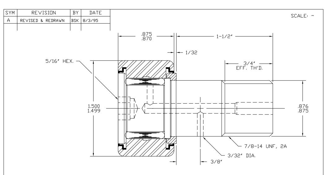
BASIC DYNAMIC CAPACITY - 4450 MAX. ALLOWABLE LOAD - 5500
