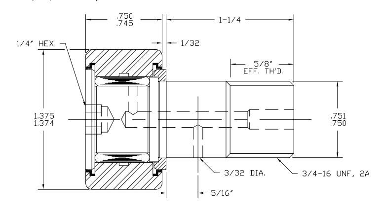
BASIC DYNAMIC CAPACITY - 3390 MAX. ALLOWABLE LOAD - 4000
