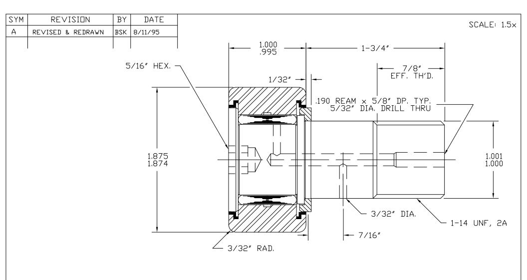
BASIC DYNAMIC CAPACITY - 6070 MAX. ALLOWABLE LOAD - 5400
