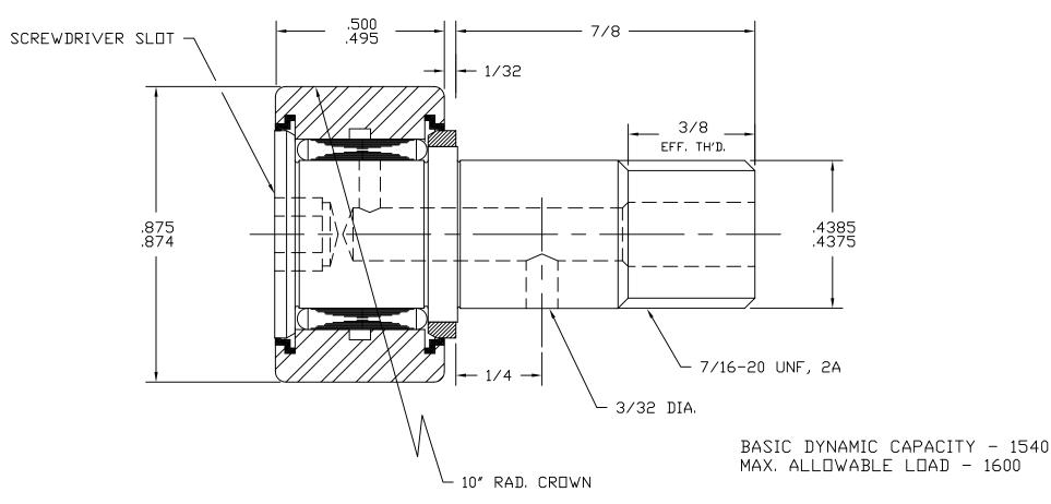
MAT'L: ST'D BEARING STEELS, SEALS-NONMETALIC. BEARING PACKED WITH GENERAL PURPOSE EP GREASE. RELUBE PROVISIONS WILL ACCEPT 3/16" DRIVE TYPE FITTINGS, PLUGS SUPPLIED FOR UNUSED HOLES. TOLERANCES
