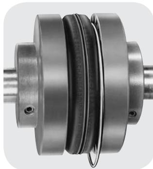
**4** Slide the loose flange on the shaft until the sleeve is completely seated in the teeth of each flange. (The "G<sub>1</sub>" dimension is for reference and not critical.) Secure the flange to the shaft. Different coupling sleeves require different degrees of alignment precision. Locate the alignment values for your sleeve size and type in the table.
