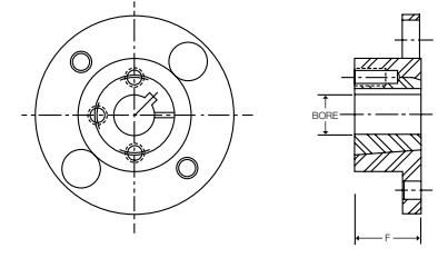
**AC/AD CLAMPING HUBS** - AC HUBS PROVIDED WITHOUT KEYWAY - AD HUBS PROVIDED WITH KEYWAY - MATERIAL CLASS A OR B ONLY
