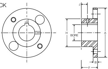
**AZ OVERSIZE BORE HUBS** - PROVIDED WITH STRAIGHT BORE AND KEYWAY
