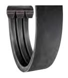
An excellent choice for narrow multiple drives where belt whip and turnover are a problem. The tie-band process assures smoother, trouble-free service. Banded belts are ideally suited for pulsating or heavily shock loaded drives and drives with long center distances.
