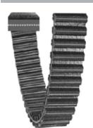
Proven performance from both sides of the belt for greater flexibility and efficiency in your drive design. Unitized process joins top and bottom teeth into one homogeneous belt with 100% rated capacity on both top and bottom side of the belt. Full fabric facing is included on all teeth.
