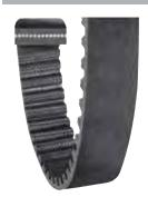
ACHE belts are designed for air-cooled heat exchangers. The belt is built with only "Z" twist cords. This gives the belt an upward direction that helps keep the belt off the bottom flanges, reducing excessive wear on the bottom side of the belt.
