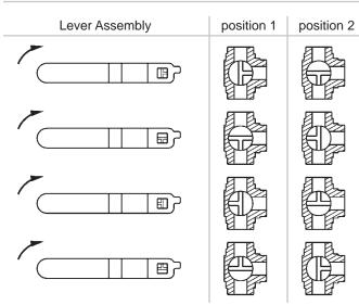
Note: 1/4 turn handle can be adjusted to any orientation. Notches on the valve stem reflect the three openings on the ball.
