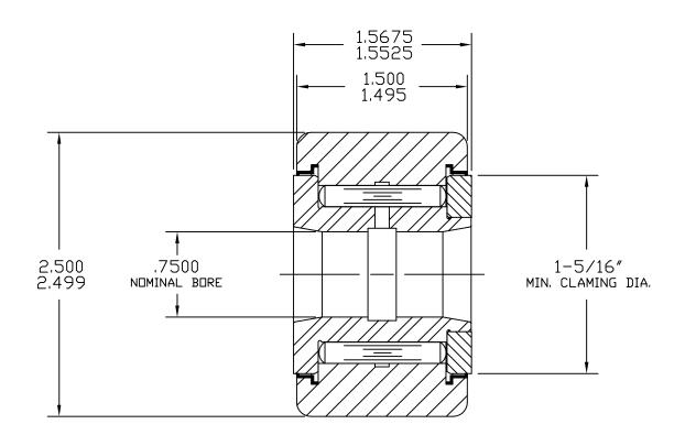
MAT'L: ST'D BEARING STEELS, SEALS - ACETAL. BEARING PACKED WITH GENERAL PURPOSE EP GREASE. RELUBE PROVISIONS WILL ACCEPT 3/16" DRIVE TYPE FITTINGS, PLUGS SUPPLIED FOR UNUSED HOLES.
