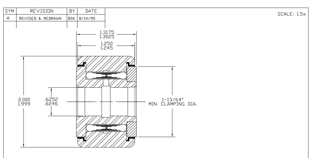
BASIC DYNAMIC CAPACITY - 8010 MAX. ALLOWABLE LOAD - 7400
