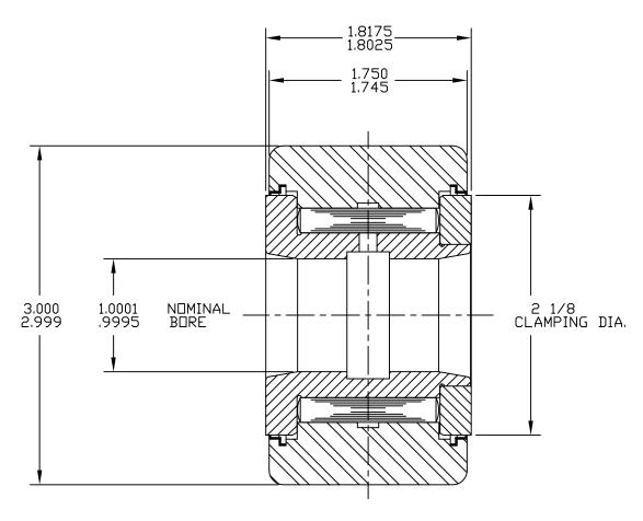
BASIC DYNAMIC LOAD RATING - 20,220 LBS BASIC STATIC LOAD RATING - 33,220 LBS
