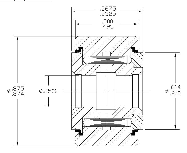
MAT'L: STAINLESS STEELS, SEALS - ACETAL, BEARING PACKED WITH GENERAL PURPOSE EP GREASE. RELUBE PROVISIONS THRU BORE.
